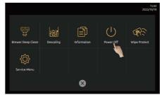
Step 3: The screen pop-up prompts. Are you "power off", click "OK" machine turns to power off mode,click"Back"to cancel this operation, the screen is off but light is still on(press the screen more than 3 seconds to wake up the machine)
