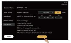
√ Grinding calibration complete.
