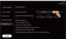
Step 5: When the device finishes taking powder at one time, take out the dregs container and weigh the powder, then clear it and put it back;
