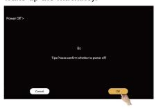
Step4: Take out the grounds container, press the power switch in the lower right corner, turn off the power, and then put it back in place. Note: Do not power off the machine directly in the startup state, so as not to cause damage to the machine.
