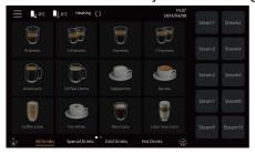
Step 6: After the system is heated, enter the quick quick rinse selection interface, If no operation is performed within 10 seconds, quick cleaning is performed by default. When finished, the main screen will be displayed.
