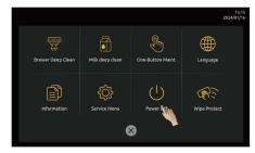
Step 3: The screen pop-up prompts. Are you "power off", click "OK" machine turns to power off mode, click "Cancel" to cancel this operation, the screen is off but light is still on (press the screen more than 3 seconds to wake up the machine).
