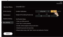
Step 5: When the device finishes taking powder at one time, take out the dregs container and weigh the powder, then clear it and put it back;
