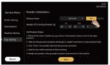
Step 6: When the device finishes taking powder at one time, take out the dregs container and weigh the powder, then clear it and put it back;
