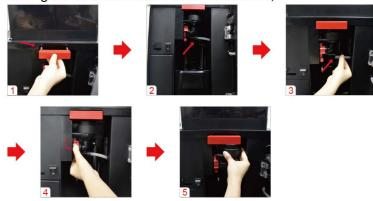
Step 3: Remove the slag container and place it on the electronic scale for zeroing and then put it back;
