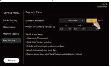
Step 8: Click the Save button to complete the current bean mill grind calibration.
