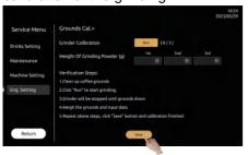
√ Grinding Calibration complete
