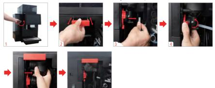
Step 2: Hold the handle as shown in the figure to push the locking device in, until it stops, then close the coffee machine door.
