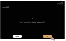
Step 4: In the state of soft shutdown, turn the key counterclockwise as shown in the figure, open the door of the coffee machine, press the power switch to completely cut off the power of the coffee machine, and lock the door. Note: Do not directly cut off the power in the power-on state to avoid damage to the machine.
