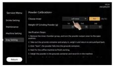
Step 8: Extract the water storage tray as shown in the figure and remove the slag box. Weigh the powder in the slag box and record it in the machine;
