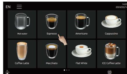
Step 2: The beverage parameter adjustment interface appears. After adjusting and confirming, click "Start Making" to proceed with the beverage (Only work under adjustable mode)
