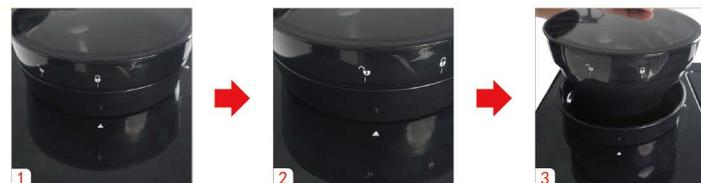
Install the bean hopper: put the bean hopper on the coffee machine installation place, make the arrow point to the unlock position, then hold the bean hopper with both hands (avoid touching the black part under the bean hopper) and rotate clockwise until the arrow points to the lock position.
